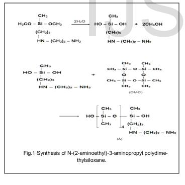
Due to this polymerization reaction the viscosity of the polymer was increased. The final product was aminomodified silicone oil polymer (B). Due to the polymerization reaction some low boiling micro molecules like  $CH_3OH$ and  $H_2O$  was remained in the reaction. After that these micro molecule was eliminated from the reaction by the vacuum distillation at  $120^{\circ}C$ .
