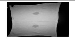
Fig.8 Treated fabric absorbency
